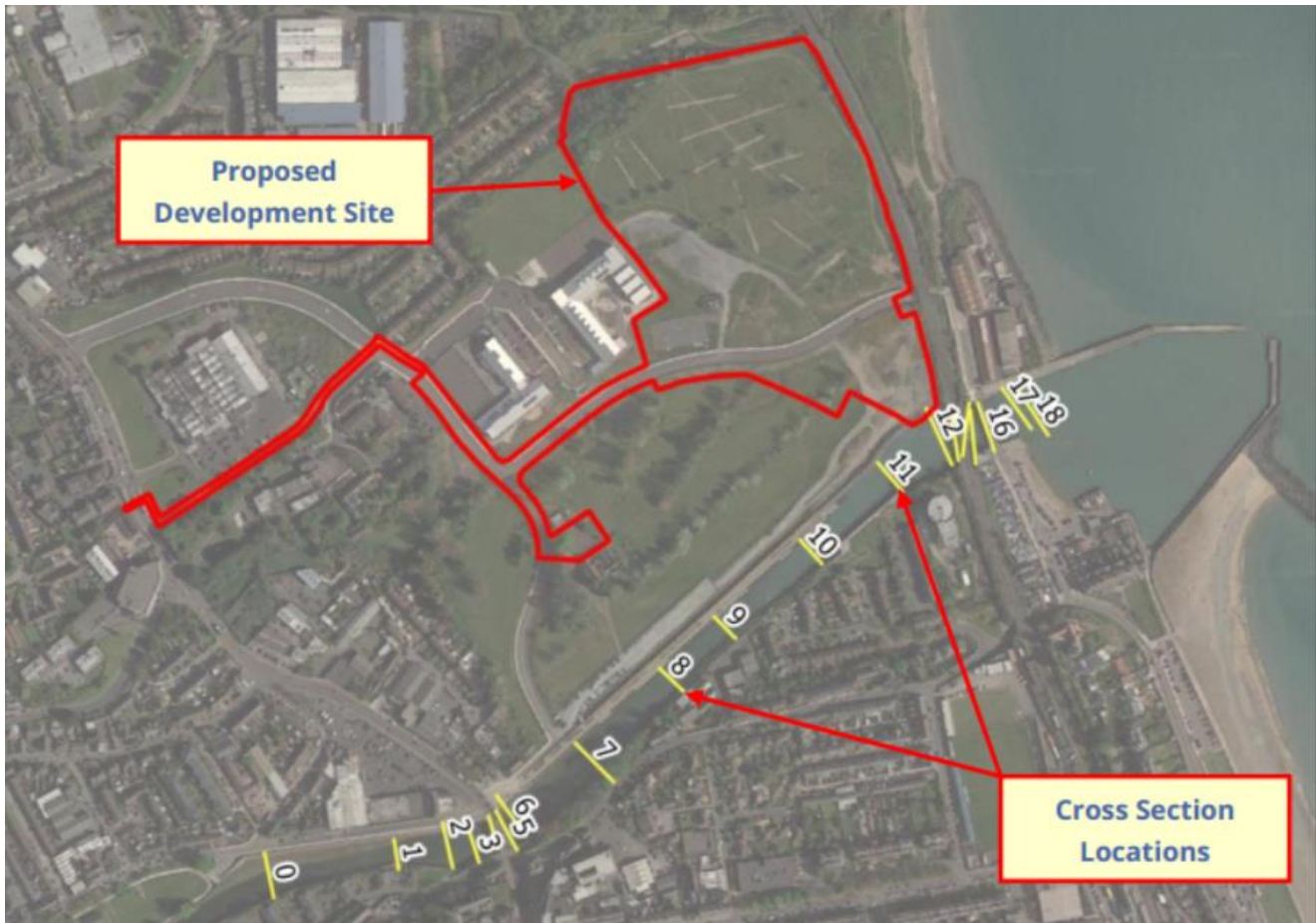
Figure 6-1 – Extents of River Model (Red line represents approximate location of the proposed site)
